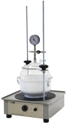
De-airing agitation device including vacuum pyknometer 75-D1123/D and electro-magnetic vibro-deareator 15-D0407/C and his device for clamping pyknometers 15-D0407/B1
